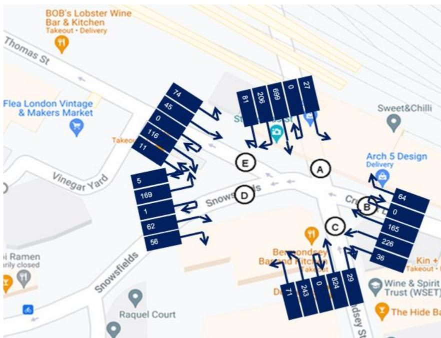
**Fig 6:** Flow diagram of cyclist movement through junction on 16 Sept 2021
